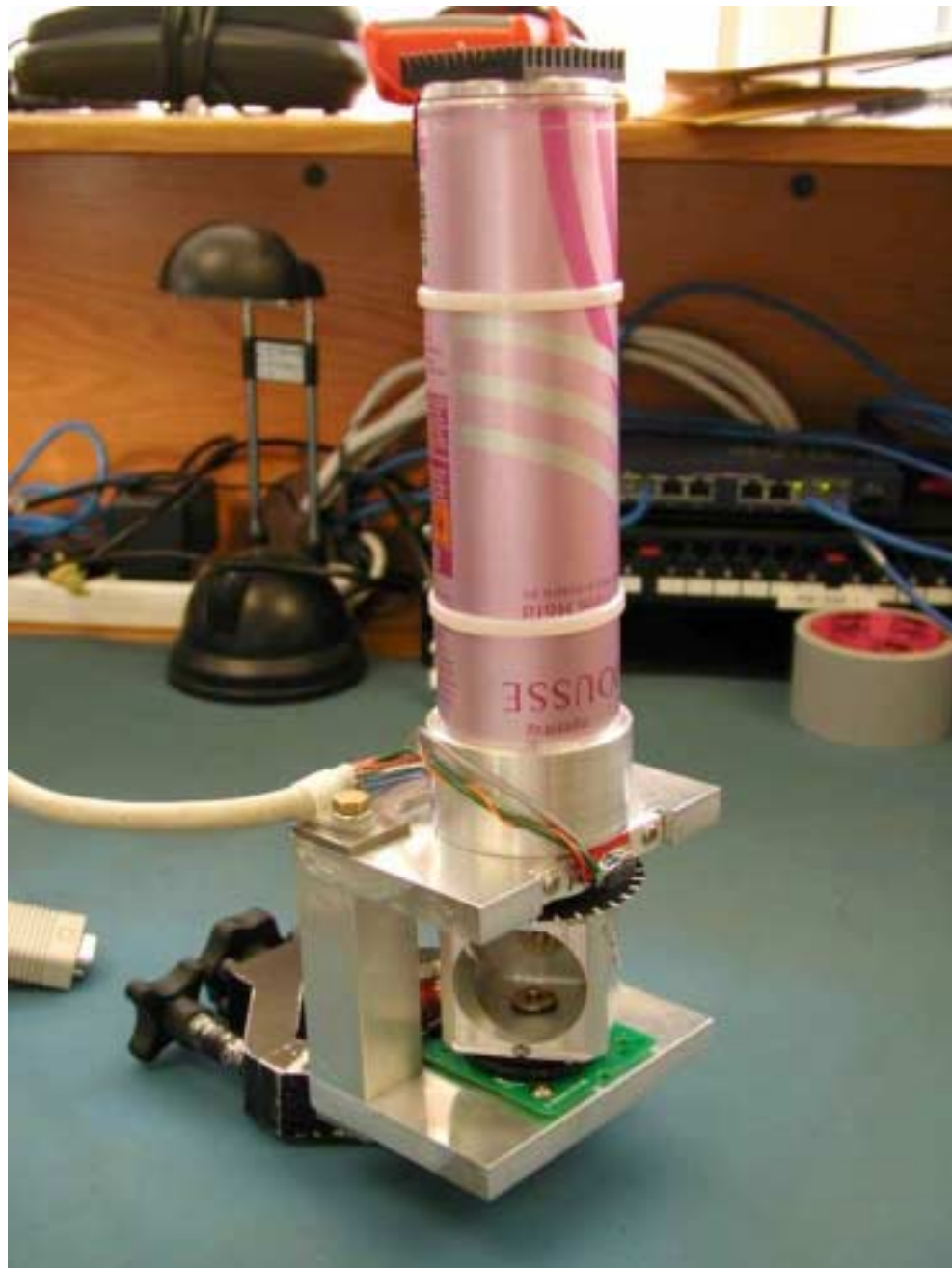
Transmitter head including mounting bracket
