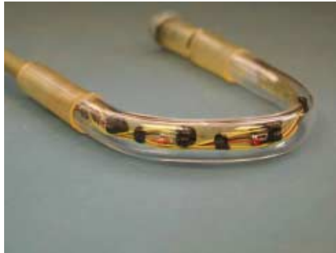
Receiver electronics in case with seals
